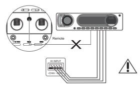
All High Level Inputs must be connected for the all channels to work properly.
