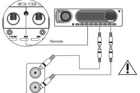
All RCA Inputs must be connected for the all channels to work properly. If the signal source is mono type, use "Y" cable at the input.
